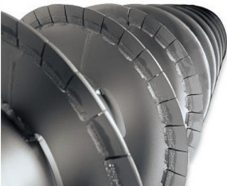
Example of the tungsten carbide tiles fitted on a Lynx decanter centrifuge
